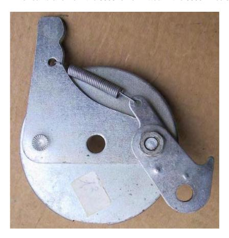
$1972\ or\ 1973$  The rotor is modified and it's dust cover is reduced from 77 to 75.5mm diameter.
