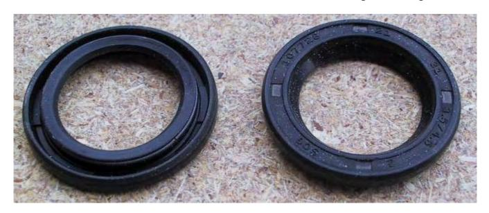
New smaller seal: 31mm OD in place of the older 40mm OD one.
