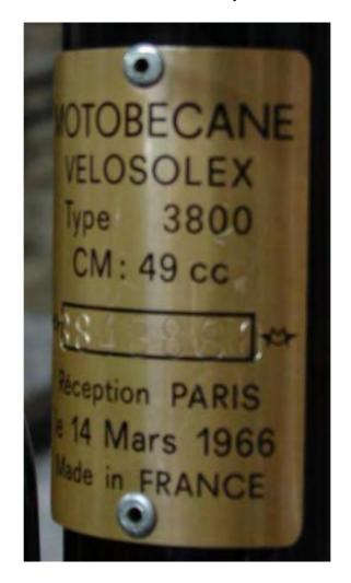
The engine numbers are now stamped onto a small aluminium label with is riveted to the crank case.
