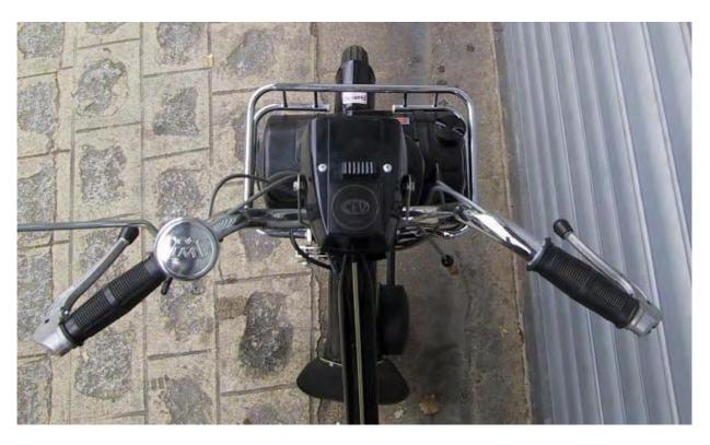
The brake levers get black rubber balls fitted to their ends.
