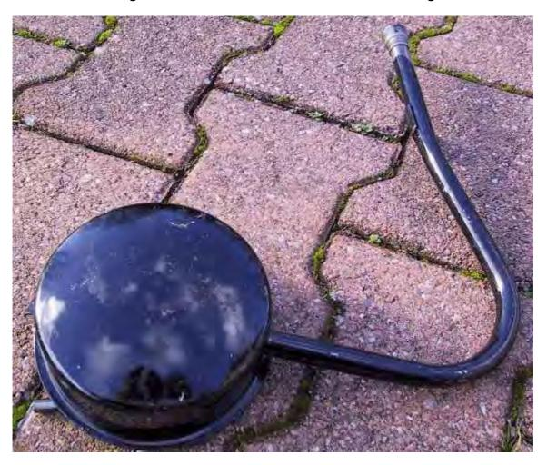
The new version of the decompression lever now has 3 holes at the control end and the control rod is lengthened by 6mm and by default fitted to the bottom hole.
