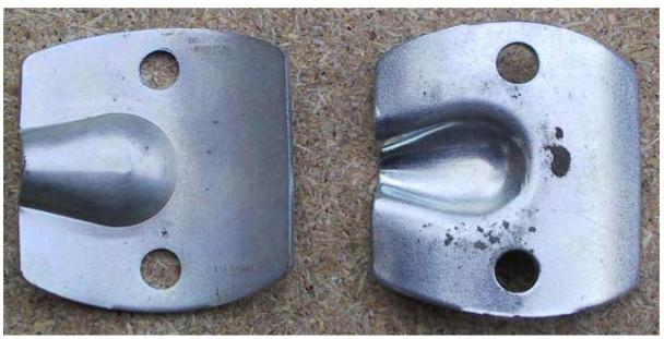
The rear mudguard is alt4ered to suit the new mounting holes required.
