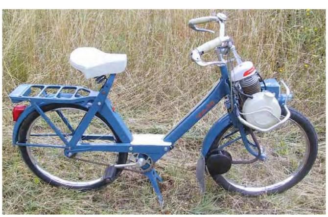
Seat cover, handle grips, footplate, flywheel cover and tank are made from light grey plastic.
