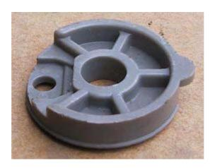
The headstem bearing nut looses its serrations, the wavy spring washer disappears and the octagonal nut is now taller.
