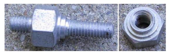
The 14mm AF Bolts on the forks are also replaced with 13mm AF ones from the 5000.
