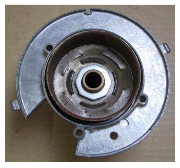
The clutch drum is secured to the friction roller with an octagonal nut of 37 mm across the flats (AF).
