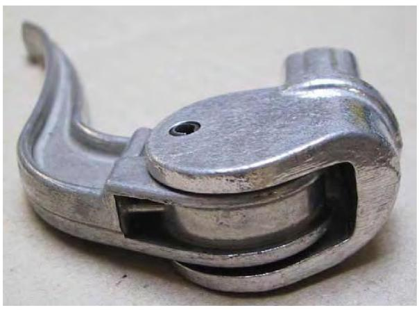
The engine cover is now fixed with a special bolt that also removes the dirt from the friction roller space, in order to make the light switch more reliable.
