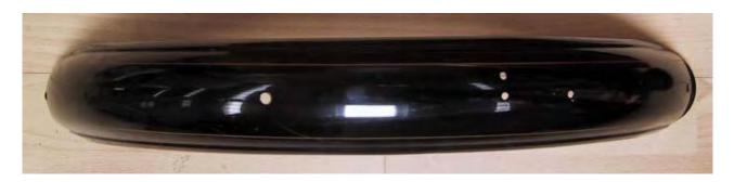
The front mudguard is extended and forms a protective shield between the exhaust gases and the mud flap.
