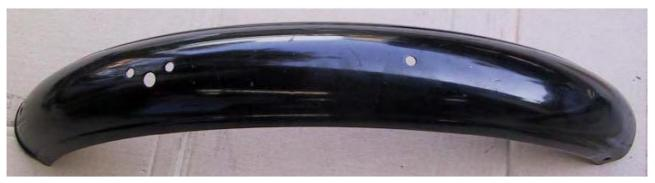
New paint produces a higher gloss. It is sprayed over a white base coat.
