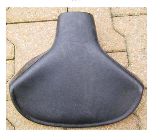
The older seat cover branded "Brown" with a line-type grain surface continues to be fitted as standard.
