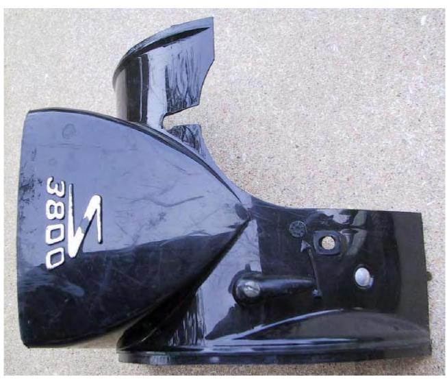
The carburettor guard is now sourced from the 5000. It has two mounting holes
