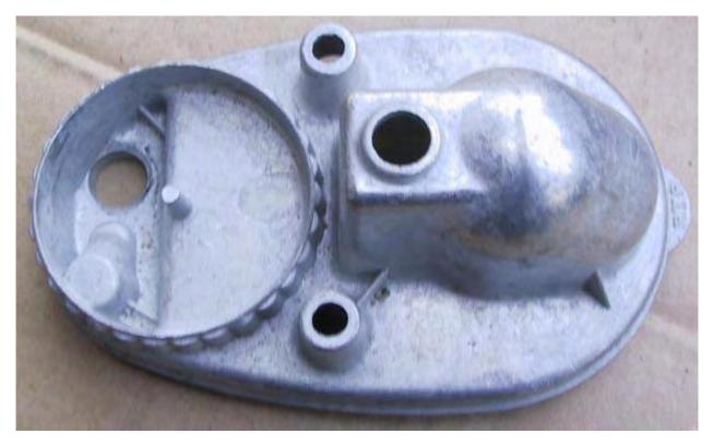
The tank lid gets a ventilation hole on both the 5000 and 3800.
